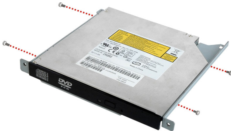
Figure 3-21: Optical Drive Screws
