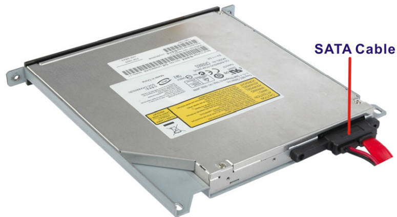
Figure 3-22: Optical Drive SATA Cable
