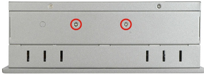
Figure 3-12: PPC-3708A-N26 HDD Bracket Retention Screws (Top Panel)
