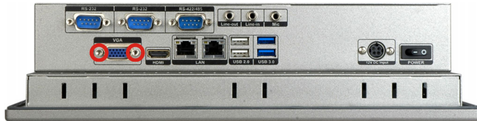
Figure 3-8: Hex Nuts on the Bottom Panel
