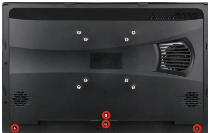
Figure 3-1: AFL3-W15B-H81 Back Cover Retention Screws
