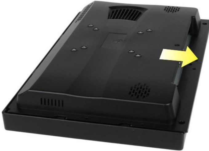
Figure 3-2: Removing the Back Cover
