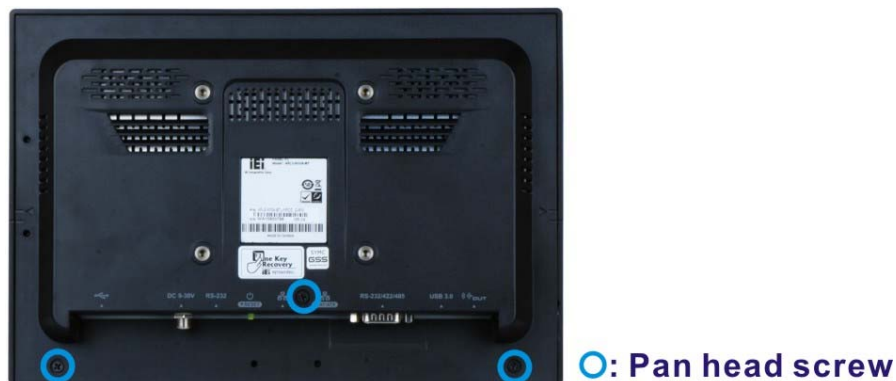
Figure 3-1: AFL3-W10A-BT Back Cover Retention Screws
