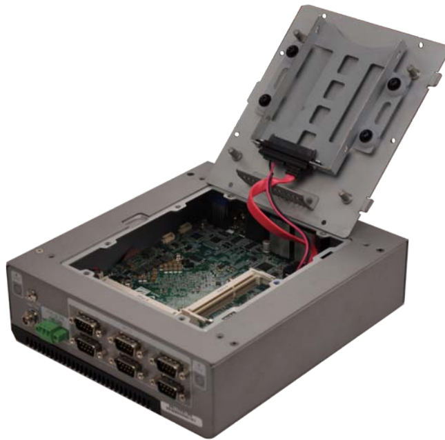
Figure 3-2: HDD Bracket Retention Screws
