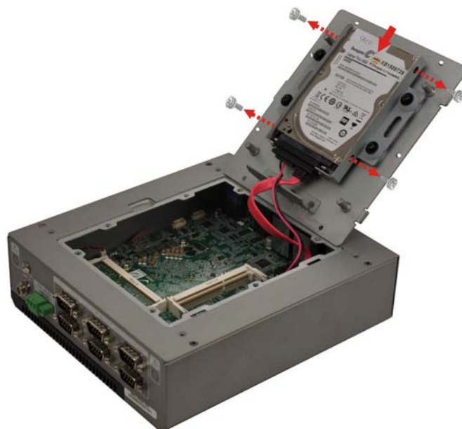
Figure 3-3: Inserting the HDD
