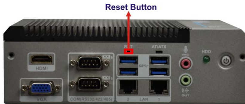
Figure 3-14: Reset Button Location
