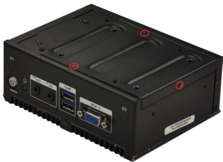
Figure 3-1: Retention Screws Removal
