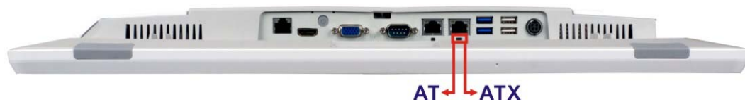
Figure 3-28: AT/ATX Switch Location
