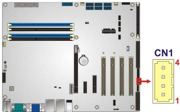
Figure 3-24: SMBus Connector Location
