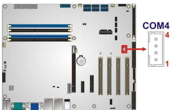
**Figure 3-23: RS-422/485 Connector Location**
