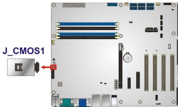
Figure 4-13: Clear CMOS Button Location
