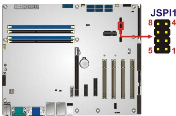
**Figure 3-25: SPI Flash Connector Location**
