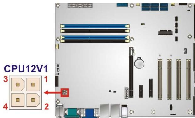
Figure 3-6: CPU Power Connector Location
