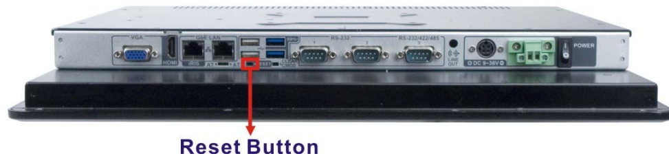
Figure 3-48: Reset Button Location
