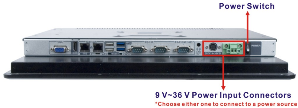
Figure 3-47: Power Connectors and Power Switch
