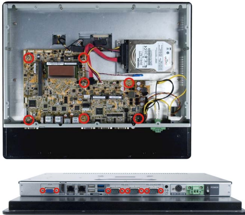
Figure 3-12: Motherboard Retention Screws
