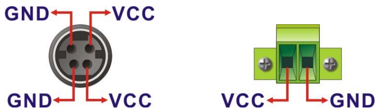
Figure 3-46: Power Input Connector Pinouts
