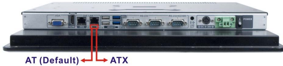
Figure 3-21: AT/ATX Mode Selection
