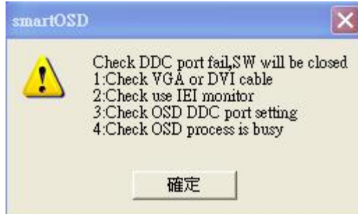
Figure C-18: DDC Port Failure
