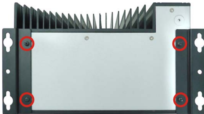
Figure 3-10: Mounting Bracket Retention Screws
