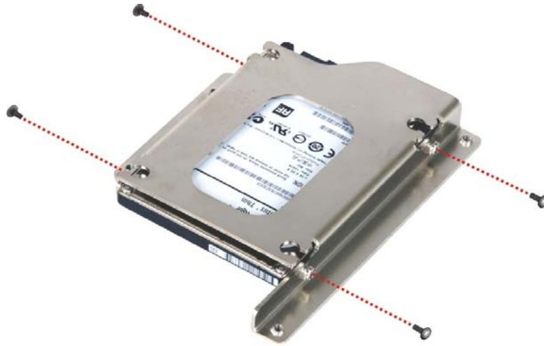
Figure 3-3: HDD Retention Screws
