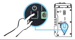
Press the power button on the front panel of the DRPC-120-QGW. It will take around 3 minutes to start up.
