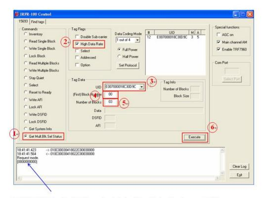
[ 00 00 00 00 00 ]: block 00~03 are all unlocked (if tag is locked, it will response 01)
