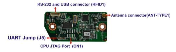
Figure 2-1: Connector and Jumper Locations
