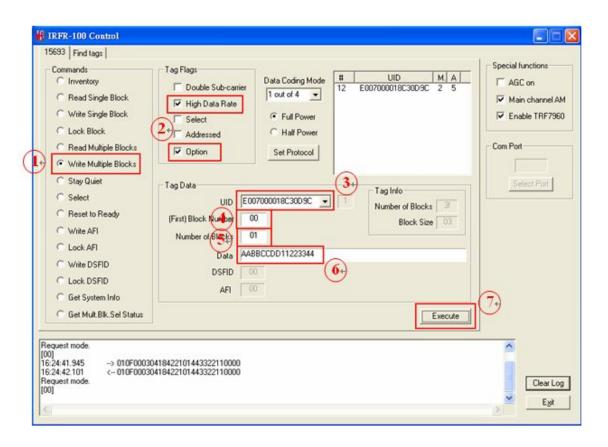
Figure 4-15: Write Multiple Block
