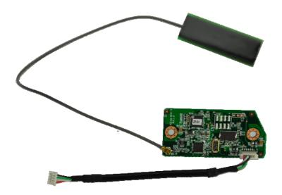
Figure 1-1: AFL2-MF-RFID-KIT Series RFID Reader
