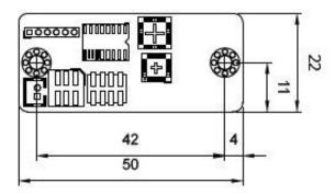
Figure 1-2: AFL2-MF-RFID-KIT Series Dimensions (mm)
