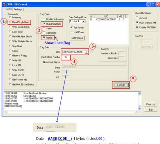
Lock Flag: 00 (fifth byte means unlocked; if 01, means locked)...
