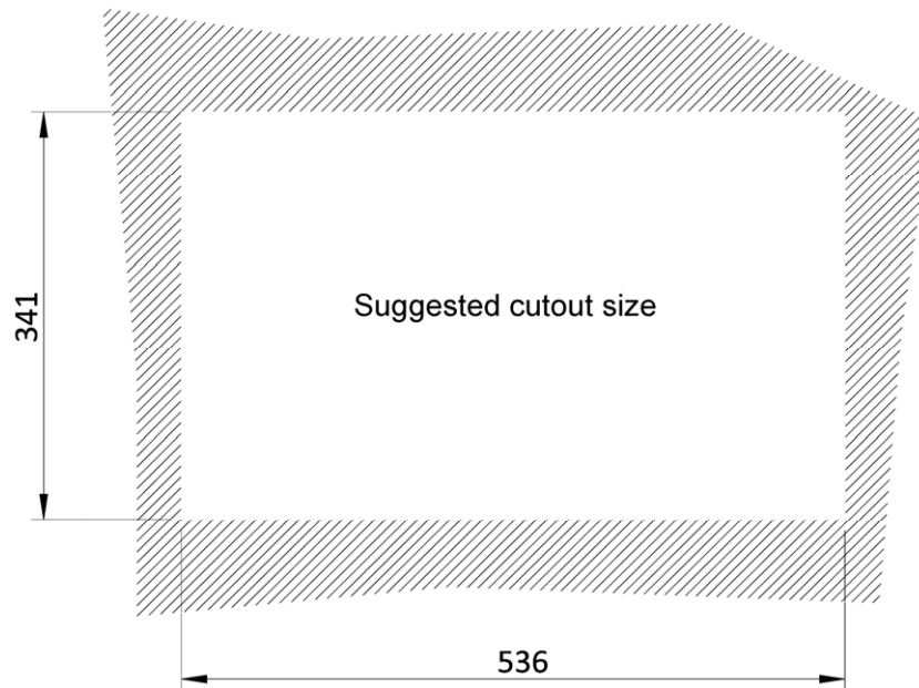
Figure 3-32: PPC-F22A-H81 Panel Cutout Dimensions
