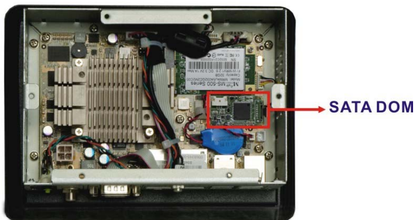
Figure 3-3: SATA DOM Installation
