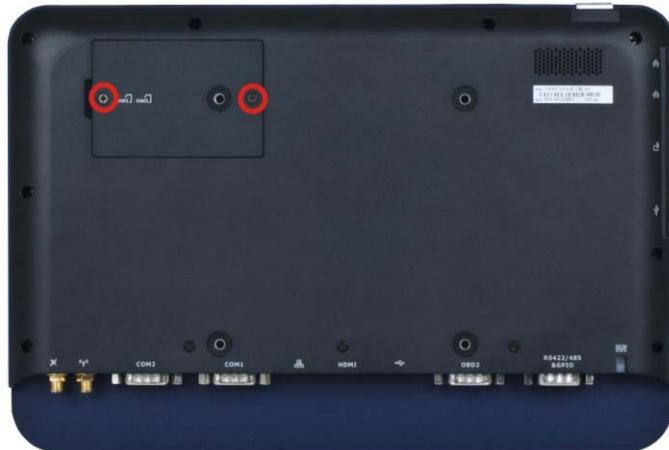
**Figure 3-3: SIM Card Slot Access Panel Retention Screws**
