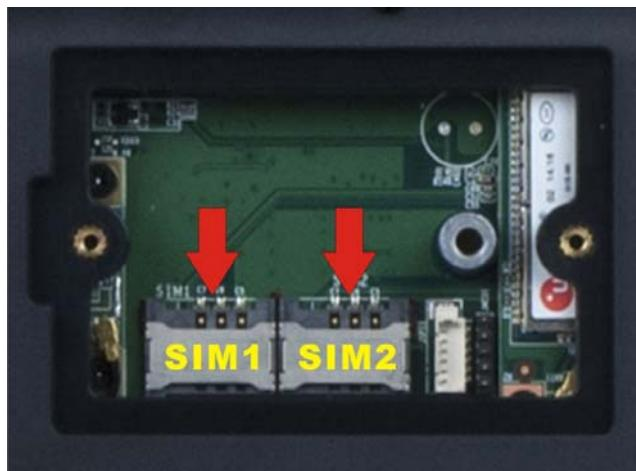
Figure 3-4: Install SIM Card
