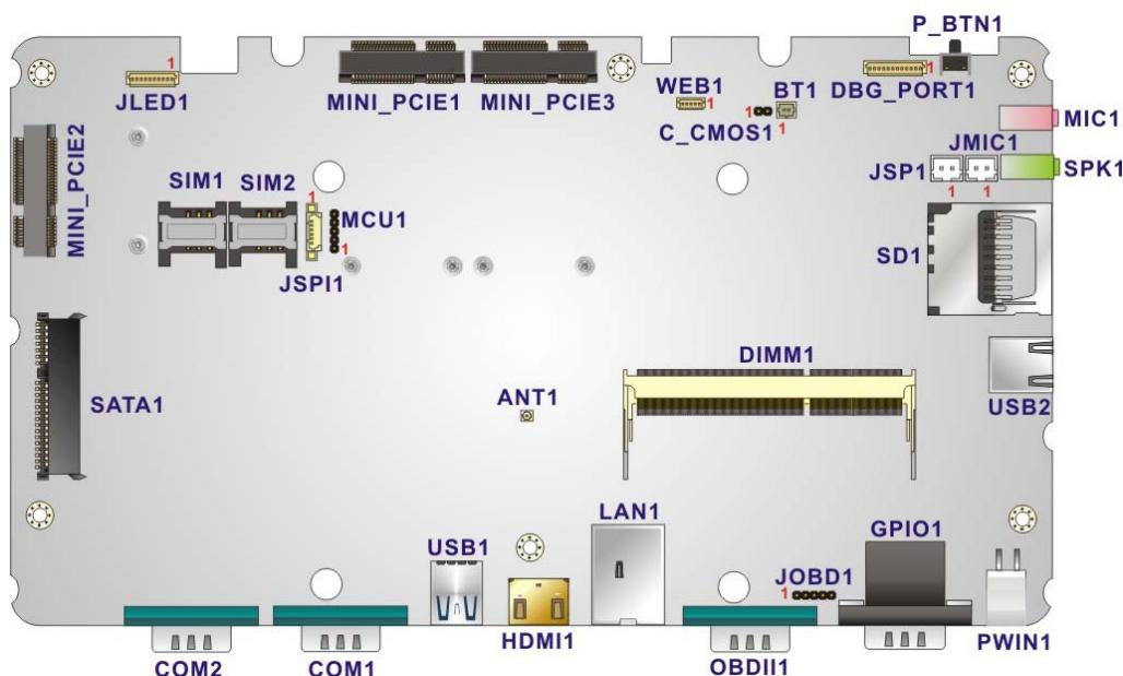
Figure 6-1: Main Board Layout Diagram (Front Side)
