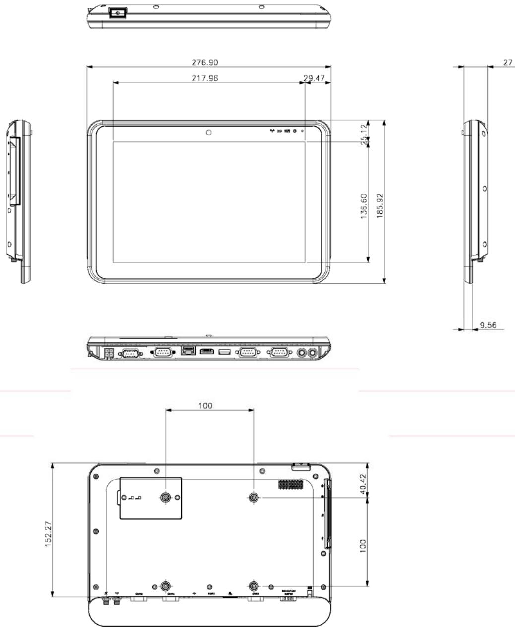
**Figure 1-8: Dimensions (unit: mm)**
