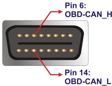
**Figure 3-10: OBD-II Connector Pinouts**
