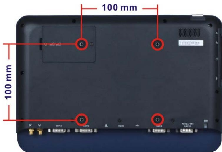
Figure 3-5: VESA Mount Retention Screw Holes
