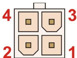
Figure 3-12: Power Input Connector
