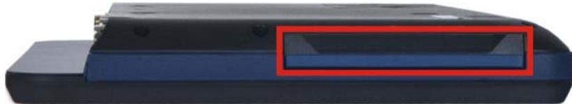
Figure 3-1: I/O Cover of the Side Panel
