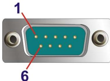
Figure 3-6: RS-232 Connector (COM1, COM2)
