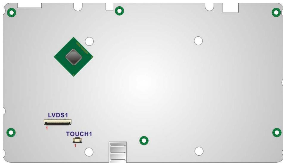
Figure 6-2: Main Board Layout Diagram (Solder Side)
