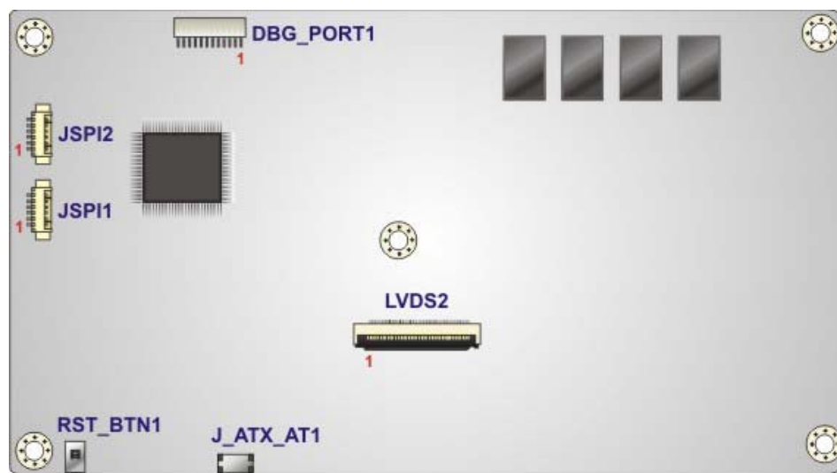
Figure 6-2: Main Board Layout Diagram (Solder Side)
