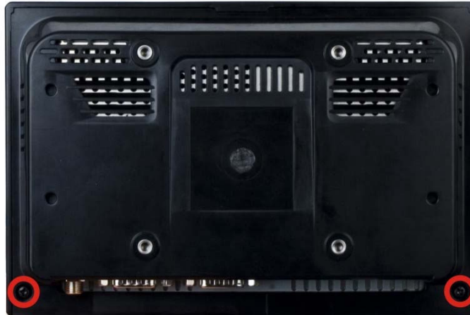
Figure 5-1: Back Cover Retention Screws
