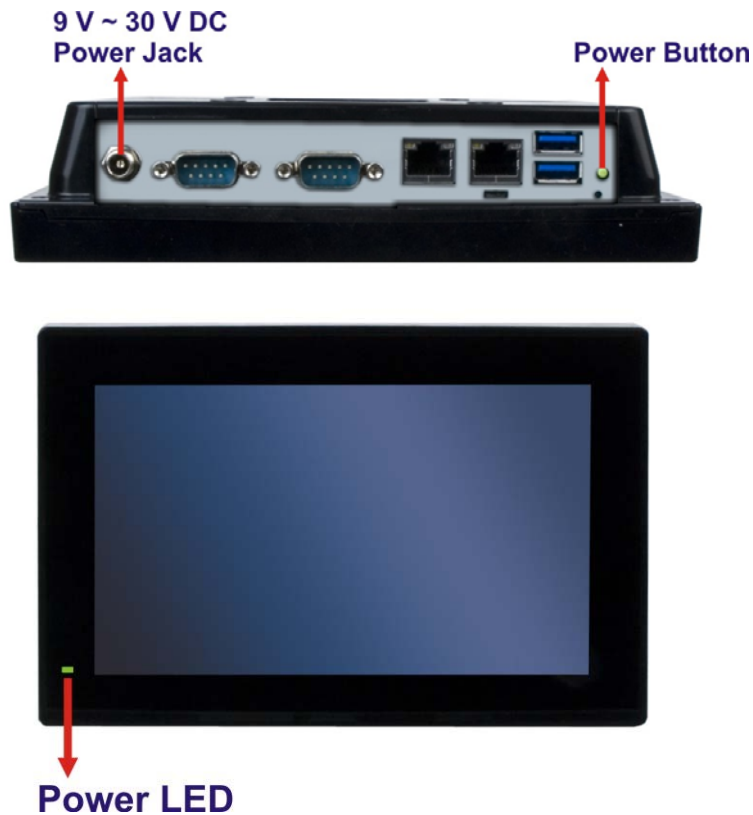
Figure 3-25: Powering On the System
