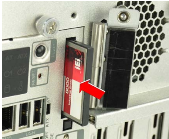
Figure 3-3: CF Card Installation
