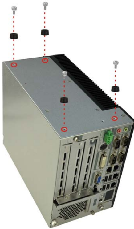
Figure 3-10: Foot Pad Installation
