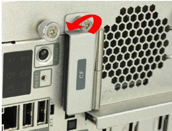
Figure 3-1: CF Card Socket
