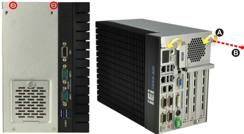
Figure 3-4: Unscrew the Cover
