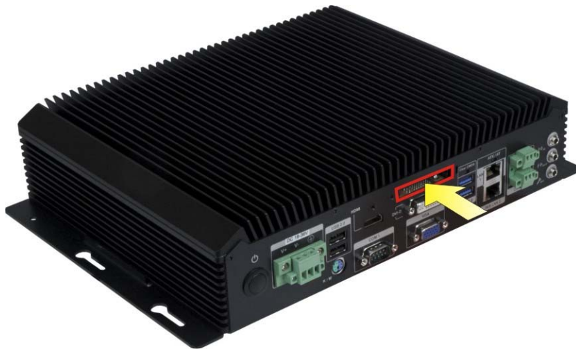
Figure 3-2: CFast Card Installation
