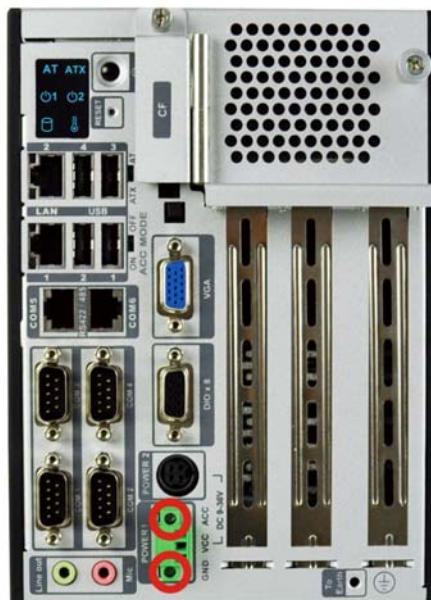
Figure 3-13: Pluggable DC-in Terminal Block Installation
