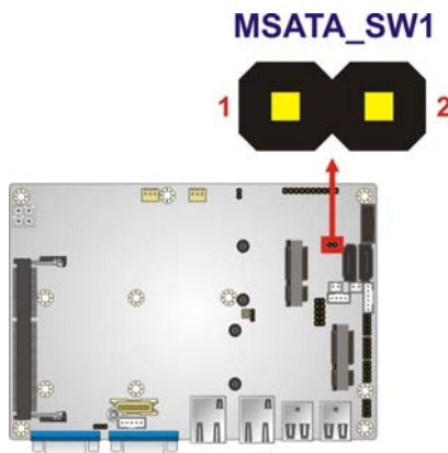
Figure 4-5: mSATA/PCIe Mini Mode Selection Jumper Location
