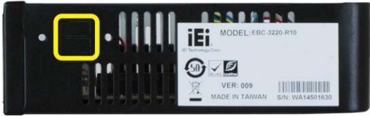
Figure 15: USB Knockout Holes
