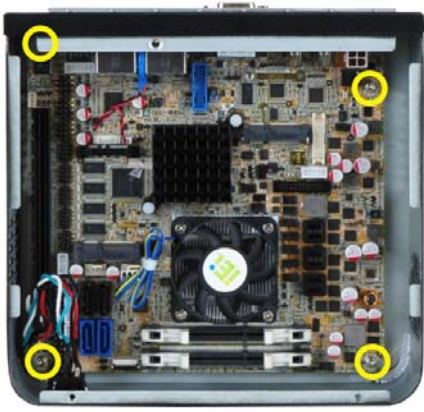
Figure 5: Motherboard Retention Screws
