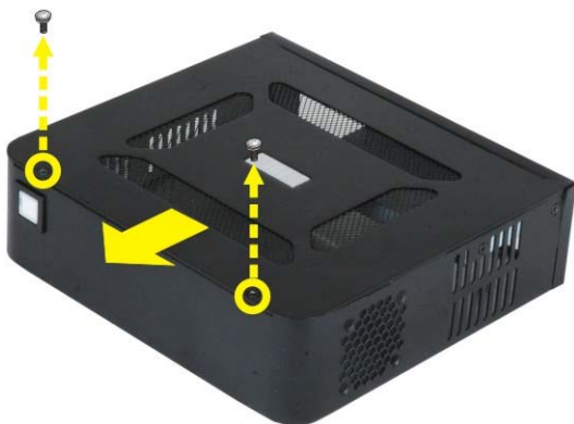
Figure 2: Top Cover Retention Screws
