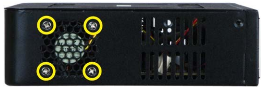
Figure 14: System Fan Retention Screws
