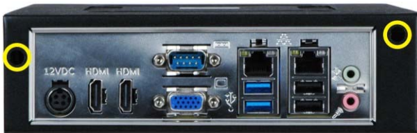
Figure 6: Knockout Holes for Wireless Antenna
