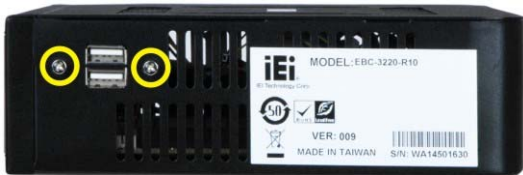
Figure 16: USB Cable Retention Screws
