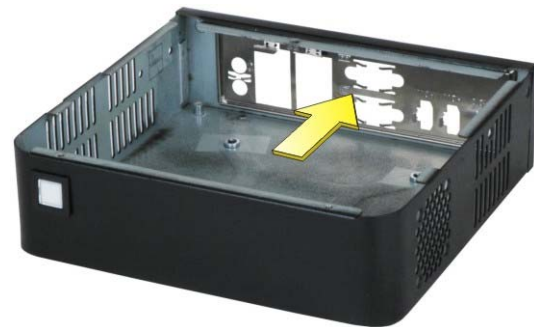
Figure 4: I/O Shielding Installation
