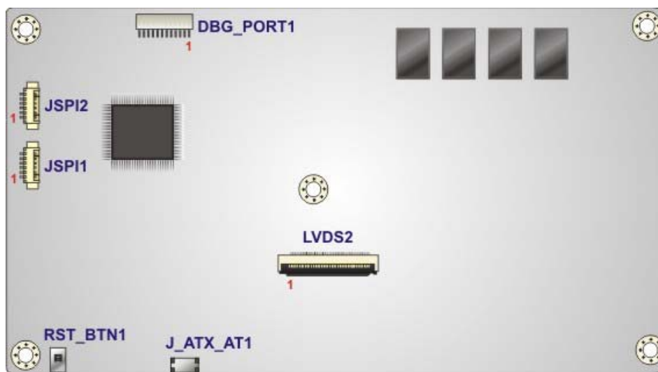
Figure 6-2: Main Board Layout Diagram (Solder Side)
