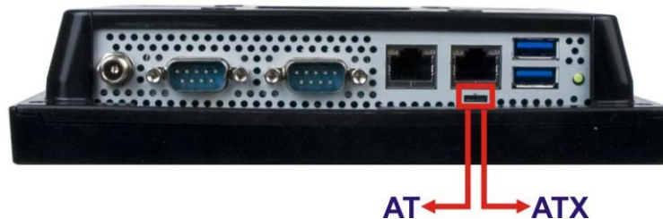
Figure 3-5: AT/ATX Switch Location
