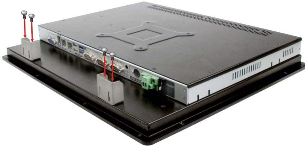
Figure 3-18: PPC-F17B-BTi Mounting Bracket Installation
