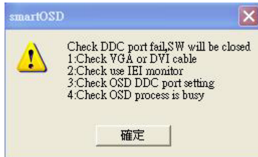
Figure C-18: DDC Port Failure
