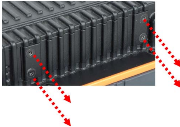
Figure 3-1: Remove the SSD Drive Bay Access Panel
