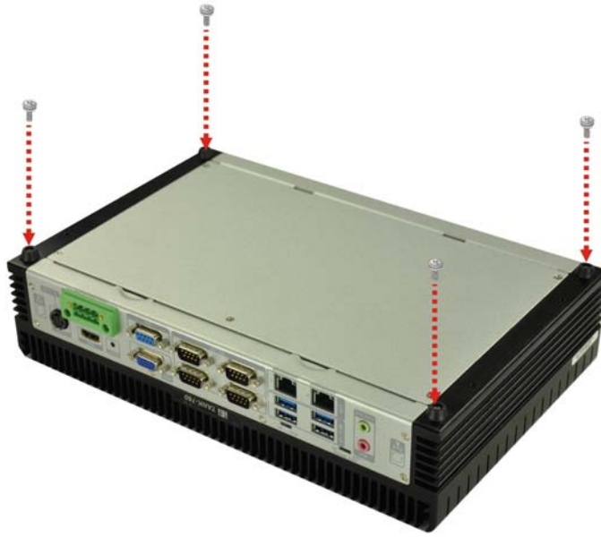
Figure 3-8: Foot Pad Installation
