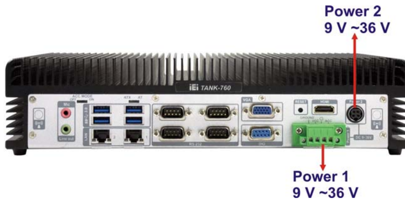
Figure 3-27: Power Connectors
