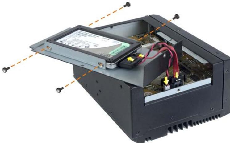
Figure 3-2: HDD Installation
