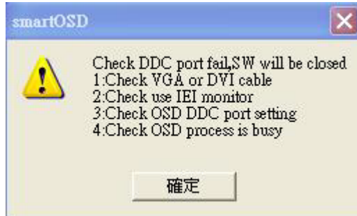
Figure C-18: DDC Port Failure
