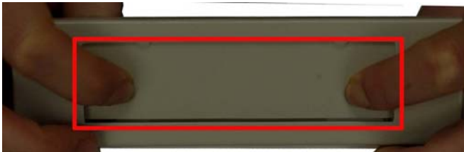
Figure 16: Bend off the front cover of the 3.5" drive bracket
