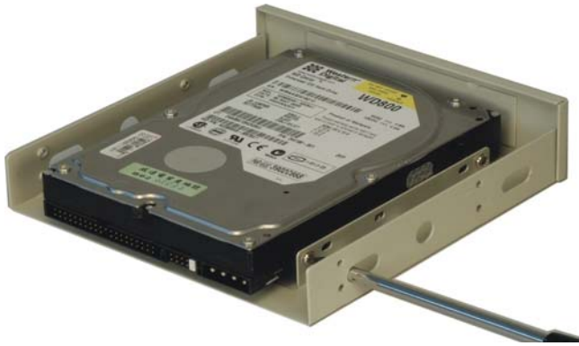
Figure 15: Install a 3.5" Disk Drive into the Adapter Bracket
