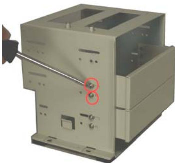
Figure 12: Remove the Front Metal Cover Retention Screws
