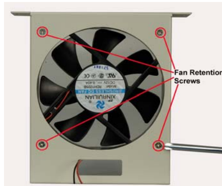
Figure 18: Remove the Fan Retention Screws
