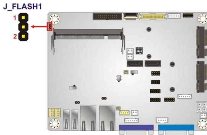
Figure 4-6: Flash Descriptor Security Override Jumper Location
