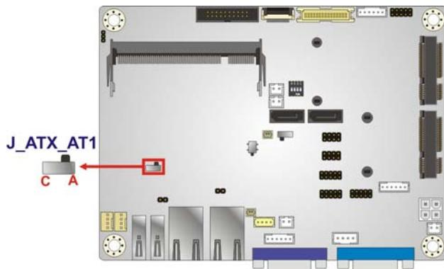
**Figure 4-2: AT/ATX Mode Select Switch Location**
