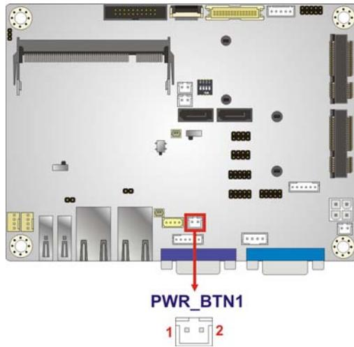
**Figure 3-17: Power Button Connector Location**
