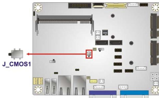
**Figure 4-3: Clear CMOS Button Location**
