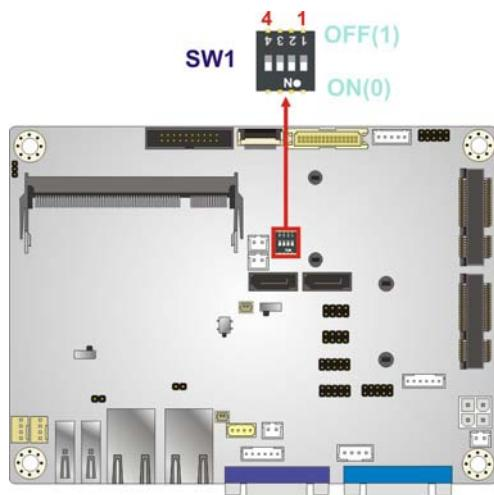
**Figure 4-4: LVDS Panel Resolution Selection Switch Location**
