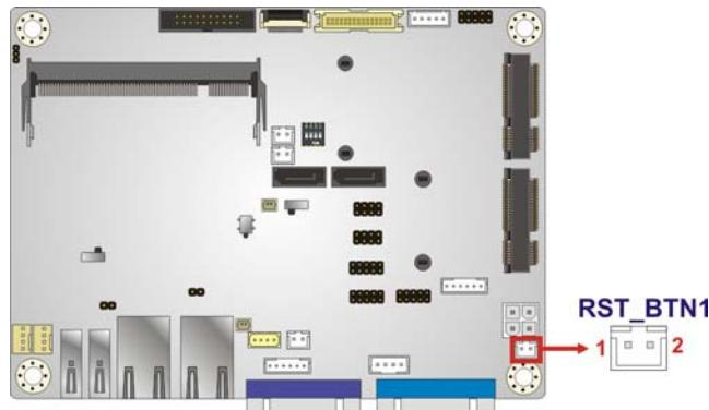
**Figure 3-18: Reset Button Connector Location**
