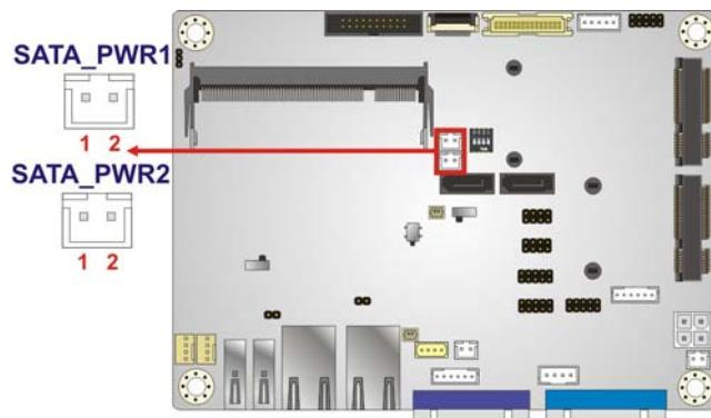
Figure 3-22: SATA Power Connector Location
