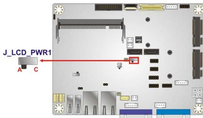
Figure 4-5: LVDS Voltage Selection Jumper Location
