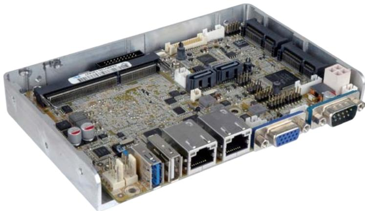
**Figure 1-1: WAFER-BT**
