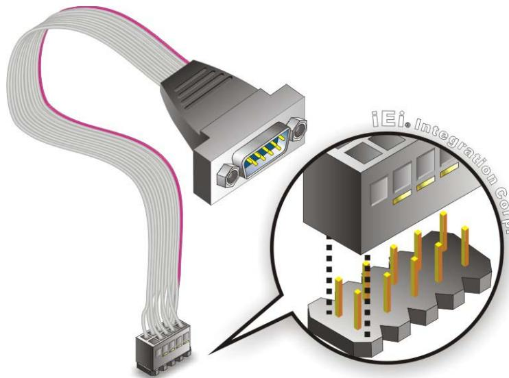
**Figure 4-9: Single RS-232 Cable Installation**
