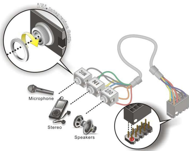
**Figure 4-7: Audio Kit Cable Connection**
