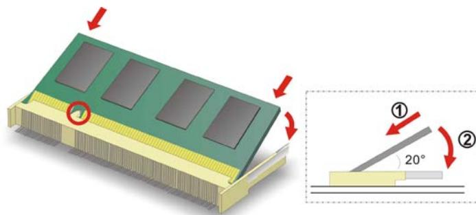
**Figure 4-1: SO-DIMM Installation**
