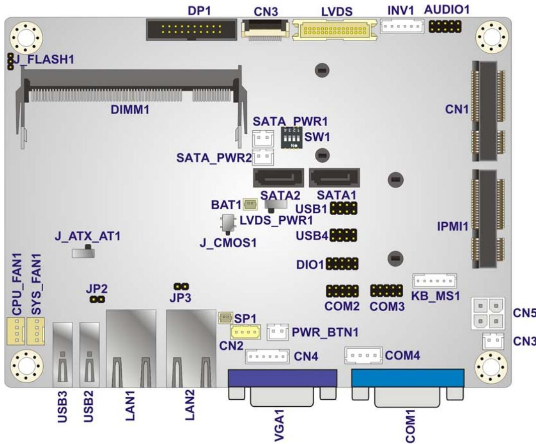
**Figure 3-1: Connector and Jumper Locations (Front)**
