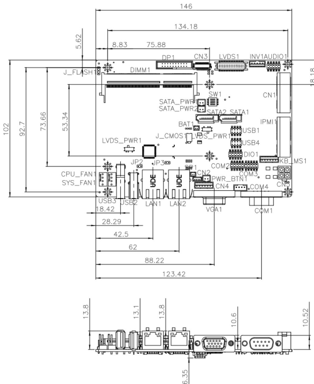
**Figure 1-3: Dimensions (mm)**
