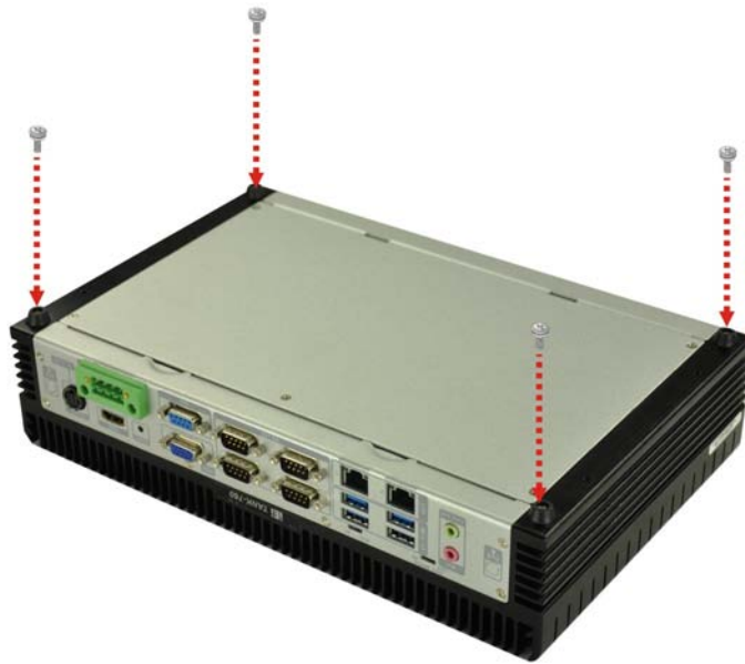
Figure 3-8: Foot Pad Installation
