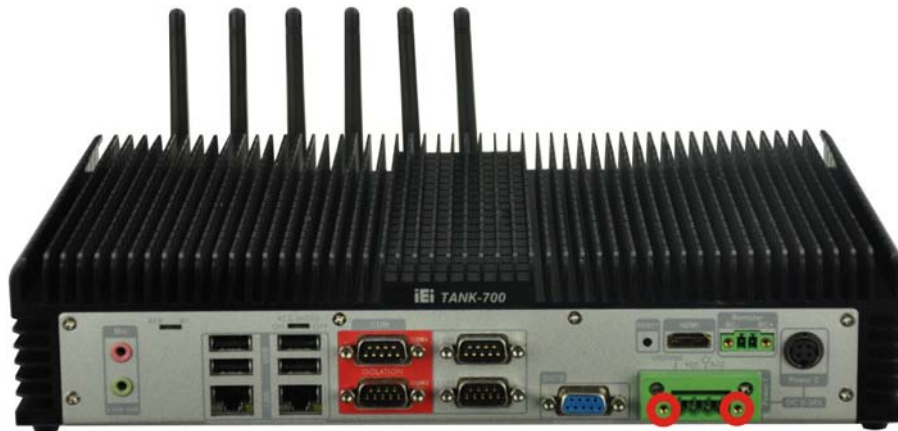
Figure 3-5: Pluggable DC-in Terminal Block Installation
