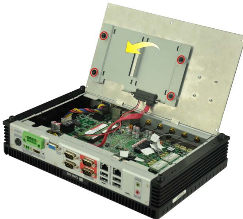
Figure 3-2: HDD Bracket Retention Screws
