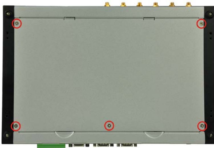
Figure 3-1: Bottom Panel Retention Screws
