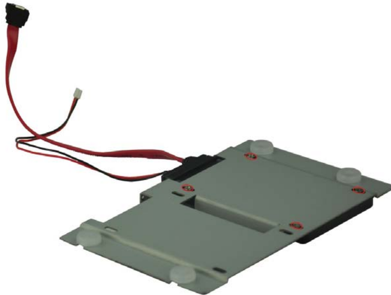
Figure 3-4: HDD Retention Screws
