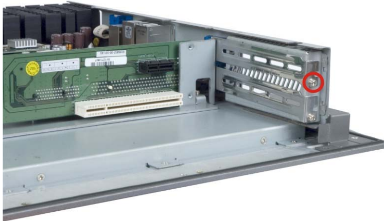
Figure 3-9: PCIe Expansion Slot Retention Screw
