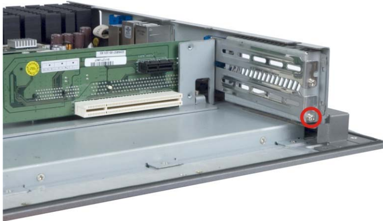
Figure 3-7: PCI Expansion Slot Retention Screw
