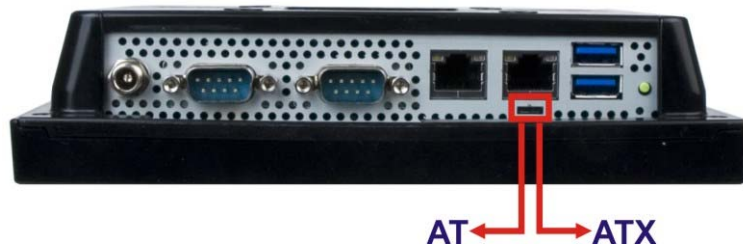
Figure 3-5: AT/ATX Switch Location
