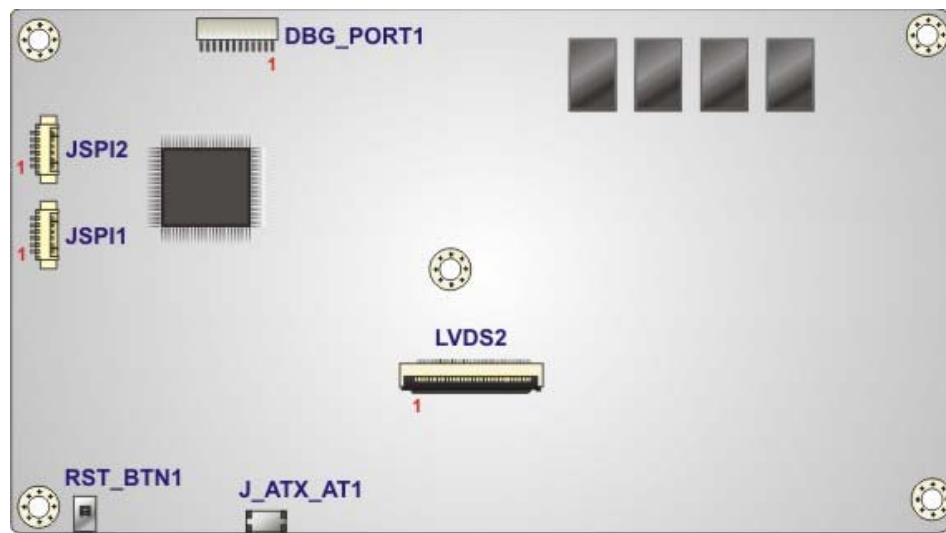
Figure 6-2: Main Board Layout Diagram (Solder Side)
