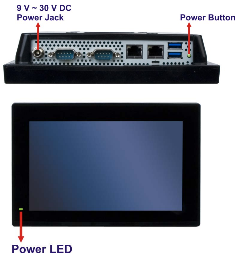
Figure 3-23: Powering On the System
