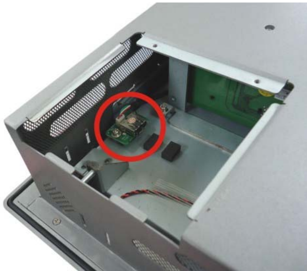
Figure 3-4: Internal USB Port Location
