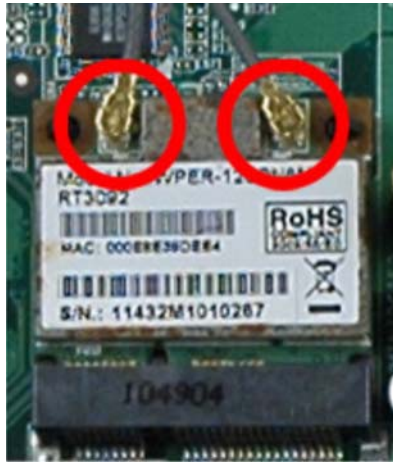
Figure 4-3: Removing the Antennas
