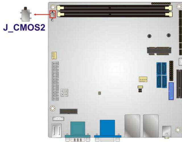
Figure 3-5: Clear CMOS Button Location
