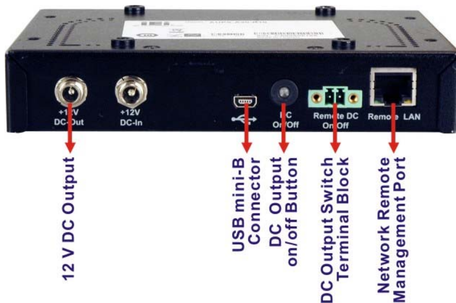
Figure 1-2: AUPS Series Standard I/O Interface Connectors
