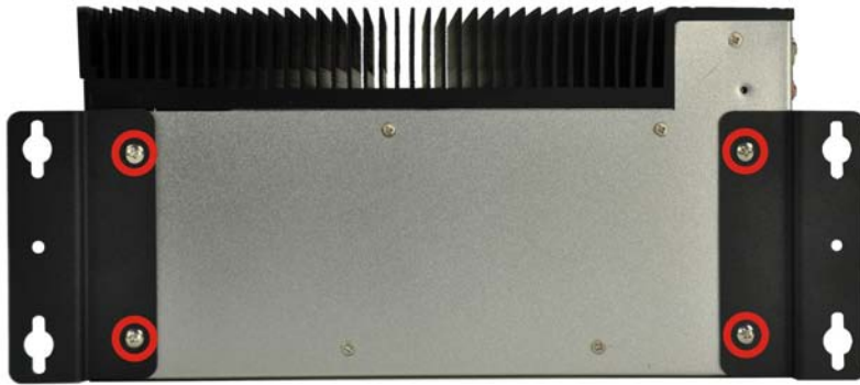
Figure 3-9: Mounting Bracket Retention Screws
