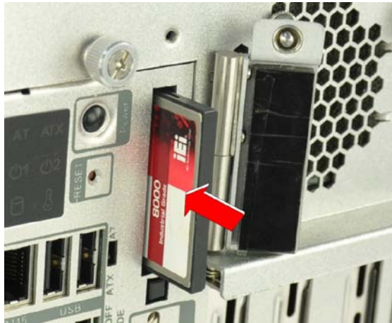
Figure 3-3: CF Card Installation
