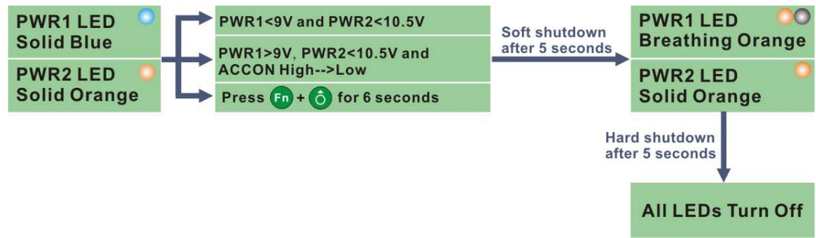
Figure 3-40: ACC On: Shutdown
