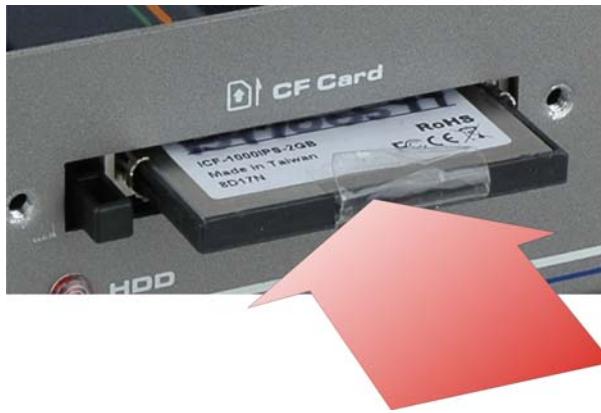
Figure 3-2: CF Card Installation
