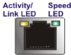
Figure 3-11: RJ-45 Ethernet Connector
