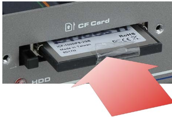
Figure 3-2: CF Card Installation
