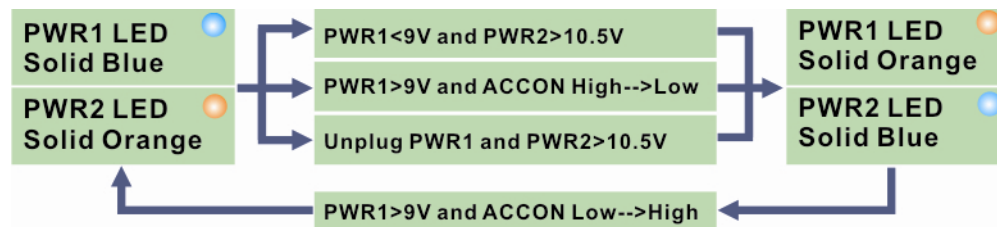
Figure 3-38: ACC On: Switch Between PWR1 and PWR2
