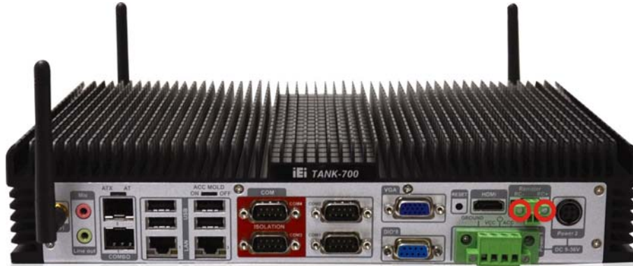
Figure 3-7: Pluggable Remote Control Terminal Block Installation
