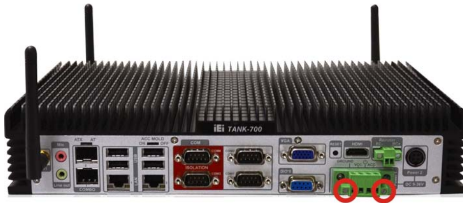
Figure 3-6: Pluggable DC-in Terminal Block Installation
