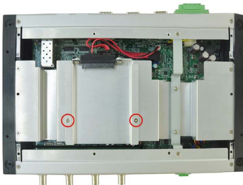
Figure 3-2: HDD Bracket Retention Screws
