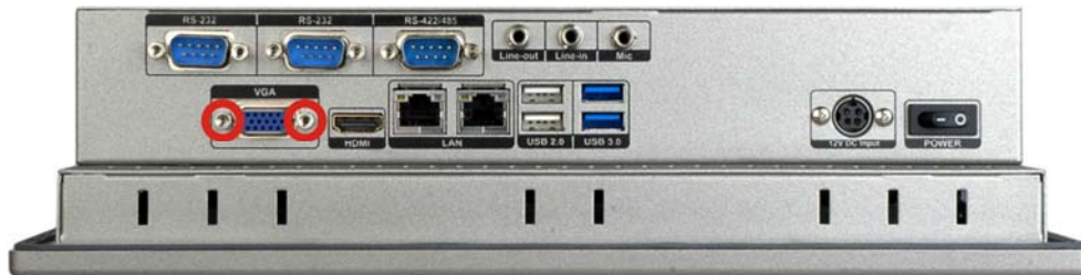
Figure 3-7: Hex Nuts on the Bottom Panel
