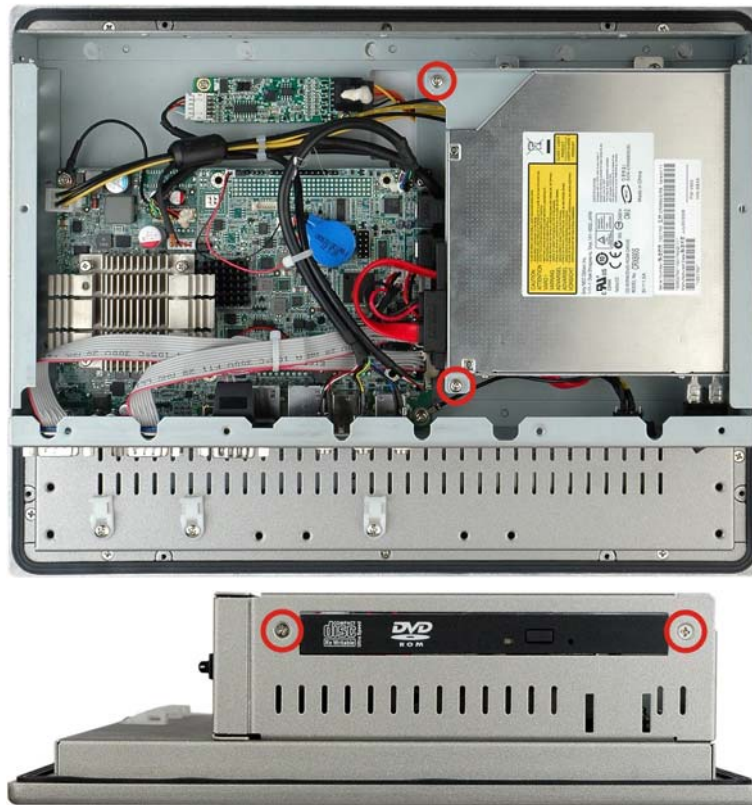
Figure 3-22: Replacing the Optical Drive Bracket
