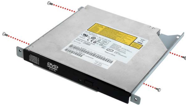
Figure 3-20: Optical Drive Screws
