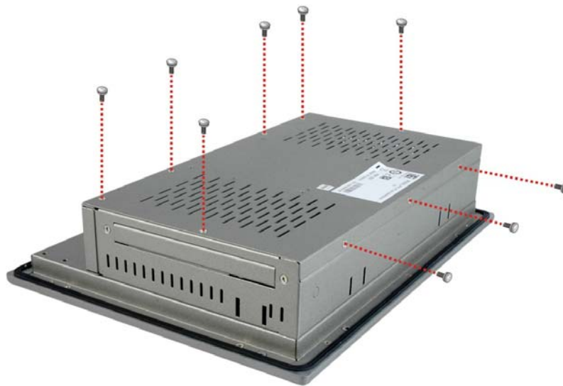
Figure 3-3: PPC-3712A-N26 Back Cover Retention Screws
