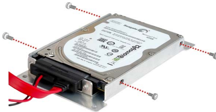
Figure 3-16: PPC-3710A-N26 HDD Retention Screws
