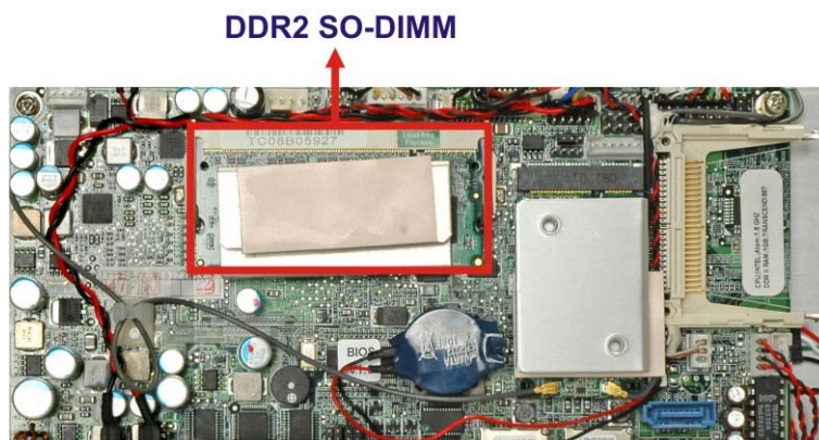
Figure 3-4: AFL-08B-N270 SO-DIMM Socket Location
