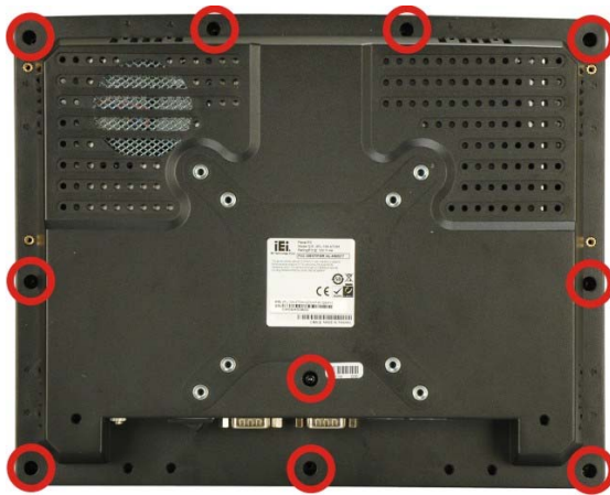
Figure 5-1: Back Cover Retention Screws
