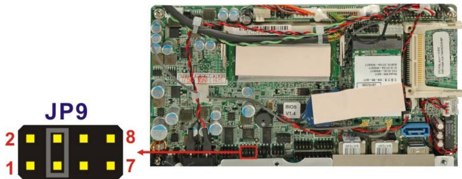
Figure 4-9: COM3 RX Function Select Jumper Location
