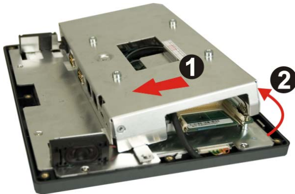
Figure 4-6: The Internal Aluminum Cover Removal
