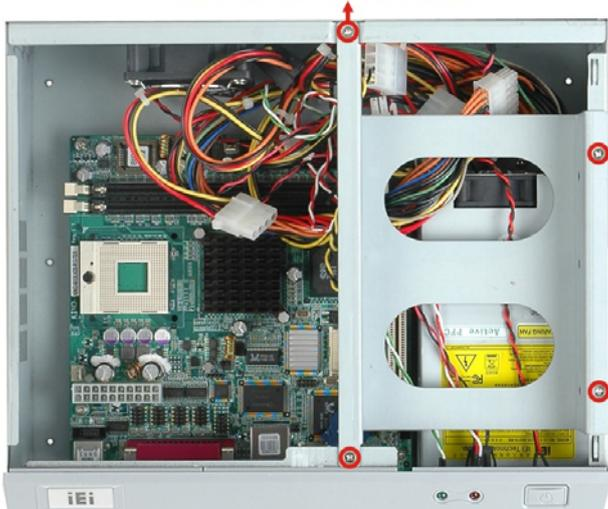
Figure 4: HDD Bracket Retention Screws
