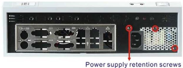
Figure 13: Power Supply Retention Screws
