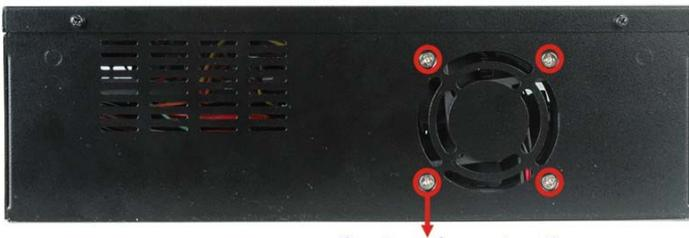
System fan retention screws
