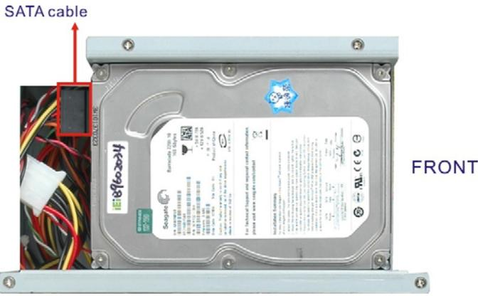
Figure 7: HDD Bracket (Top)
