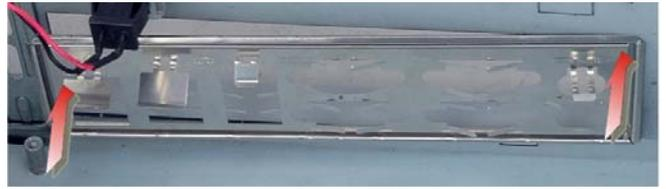
Figure 5: I/O Bracket Installation
