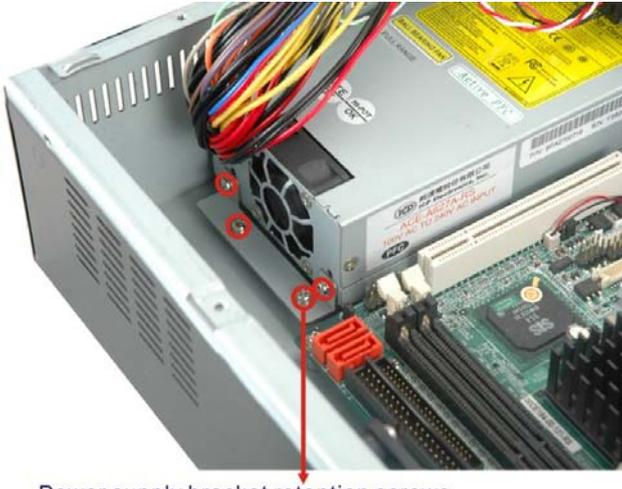
Power supply bracket retention screws
