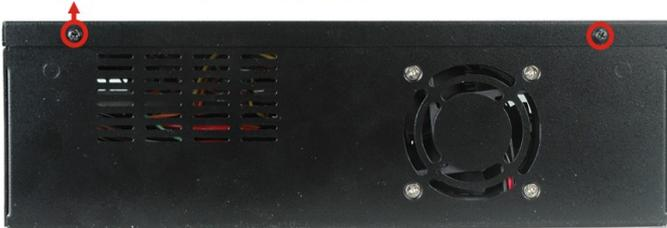
Figure 3: Chassis Cover Retention Screws
