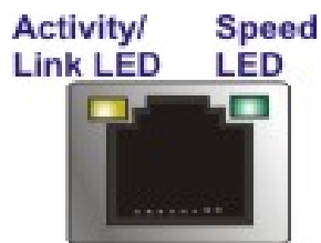
Figure 3-19: RJ-45 Ethernet Connector
