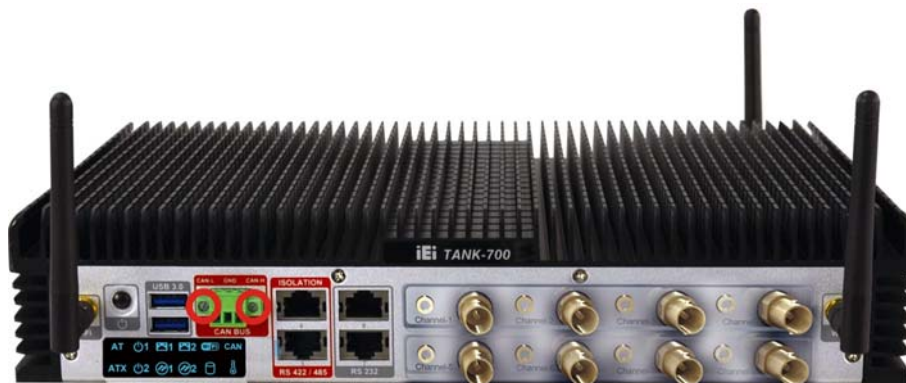
Figure 3-5: Pluggable CAN-bus Terminal Block Installation
