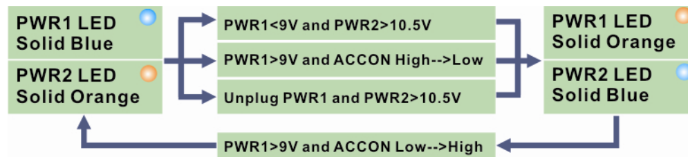
Figure 3-38: ACC On: Switch Between PWR1 and PWR2
