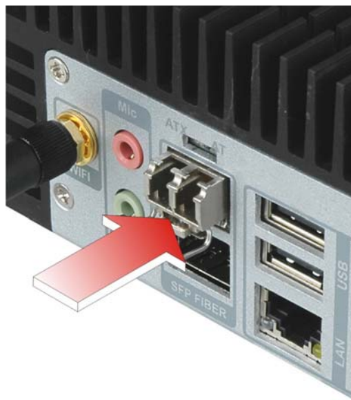
Figure 3-8: SFP Module Installation
