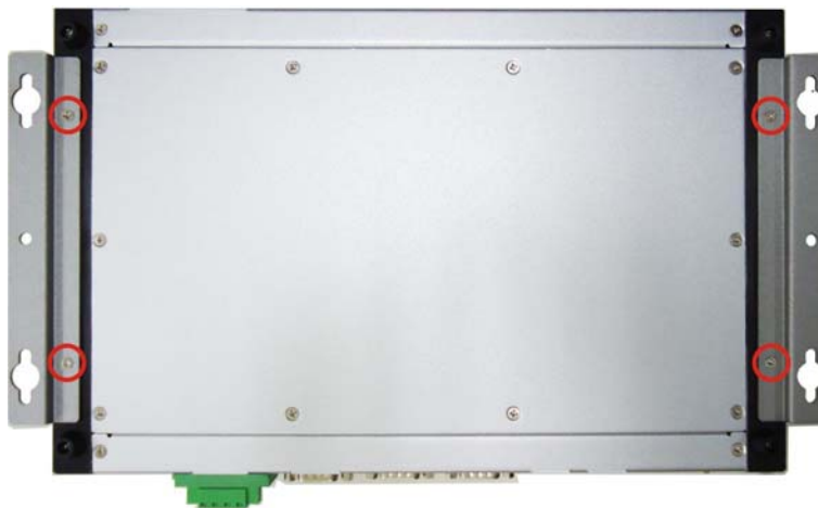
Figure 3-12: Mounting Bracket Retention Screws
