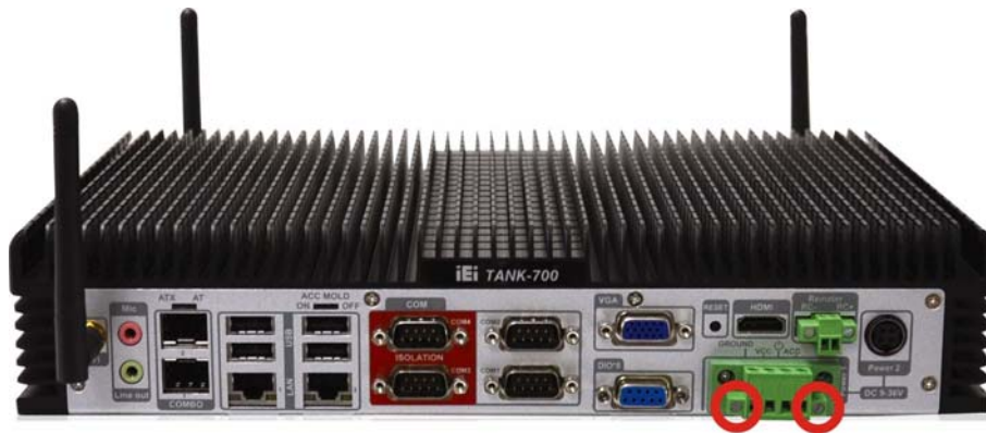
Figure 3-6: Pluggable DC-in Terminal Block Installation
