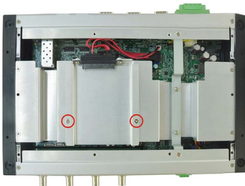
Figure 3-2: HDD Bracket Retention Screws
