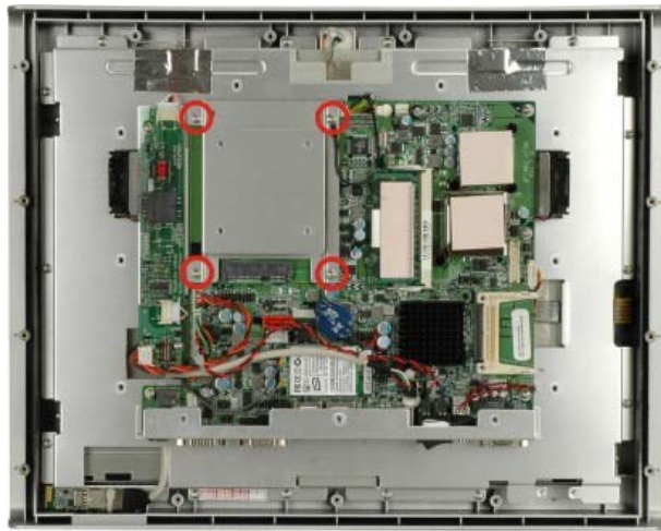
Figure 4-3: HDD Bracket Retention Screws
