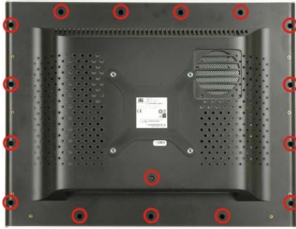
Figure 5-1: Back Cover Retention Screws
